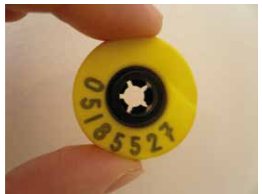
Transponder for horse identification
